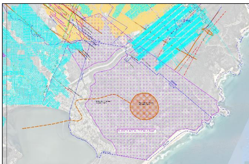
Figure 2.2: Proposed drone aerial magnetic survey over the Munmorah State Conservation Area for igneous intrusions presented in the Conceptual Project Development Plan presentation in June 2020
